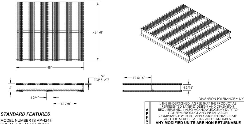
**OVERALL WIDTH IS 42 1/8" OVERALL LENGTH IS 48" OVERALL HEIGHT IS 6"** THICKNESS OF TOP SLAT IS 3/4" FLOOR (STATIC) CAPACITY: 6,000 LBS FORK (DYNAMIĆ) CAPACITY: 4,000 LBS UNSUPPORTED PALLET RACK CAPACITY: 6,000 LBS FORK OPENINGS: 19 5/16"W x 4 5/16"H
