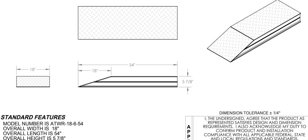
ANGLED APPROACH LENGTH IS 18" MAX UNIFORM CAPACITY IS 30,000 LBS PER PAIR (SOLD EACH) ALL WELDED ALUMINUM CONSTRUCTION
