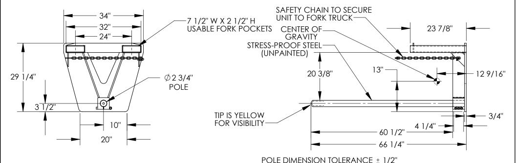
HORIZONTAL CENTER OF GRAVITY: 12 9/16" **VERTICAL CENTER OF GRAVITY: 13"**
