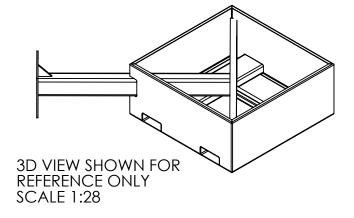
NOTE: MUST BE FILLED WITH GRAVEL OR LIMESTONE AGGREGATE CONCRETE.
