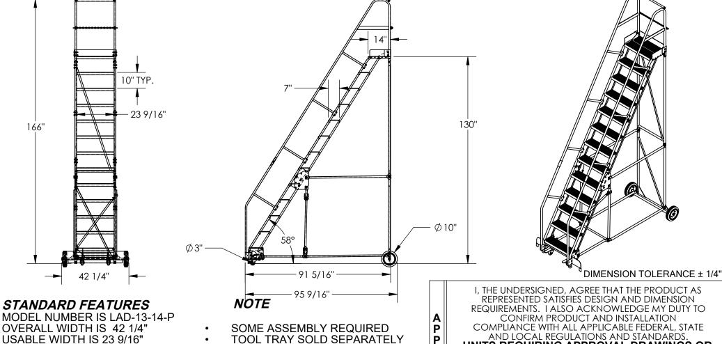
USABLE WIDTH IS 23 9/16" OVERALL LENGTH IS 95 9/16" **USABLE LENGTH IS 91 5/16" OVERALL HEIGHT IS 166"** TOP STEP HEIGHT IS 130" STEP TYPE IS PERFORATED CLIMB ANGLE IS 58° STEP DEPTH IS 7" **TOP STEP DEPTH IS 14"**
