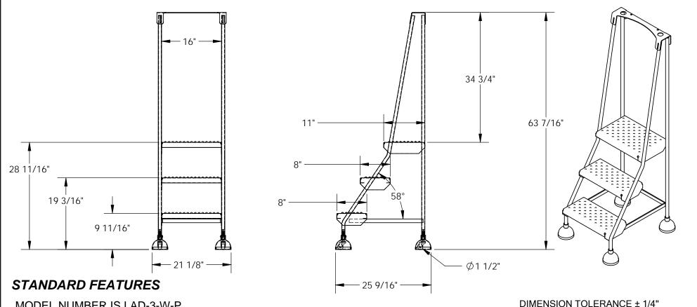
MODEL NUMBER IS LAD-3-W-P **OVERALL WIDTH IS 21 1/8" USABLE WIDTH IS 16" OVERALL LENGTH IS 25 9/16" OVERALL HEIGHT IS 63 7/16" CAPACITY IS 300 LBS** STEP TYPE: FORMED STEEL STEPS WITH PERFORATED ANTI-SLIP TOP SURFACE BOTTOM STEP HEIGHT 9 11/16" ± 1/4" TOP STEP HEIGHT 28 11/16" ± 1/4" STEP SIZES 8" X 16"
