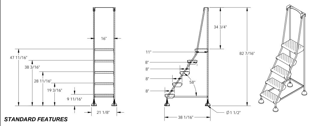
MODEL NUMBER IS LAD-5-W-P **OVERALL WIDTH IS 21 1/8" USABLE WIDTH IS 16"** OVERALL LENGTH IS 38 1/16" **OVERALL HEIGHT IS 82 7/16" CAPACITY IS 300 LBS** STEP TYPE: FORMED STEEL STEPS WITH PERFORATED ANTI-SLIP TOP SURFACE BOTTOM STEP HEIGHT 9 11/16" ± 1/4" TOP STEP HEIGHT 47 11/16" ± 1/4" STEP SIZES 8" X 16" COLOR: POWDERCOATED WHITE SPRING LOADED CASTER WITH STEEL DOME AND RUBBER PAD BOTTOM
