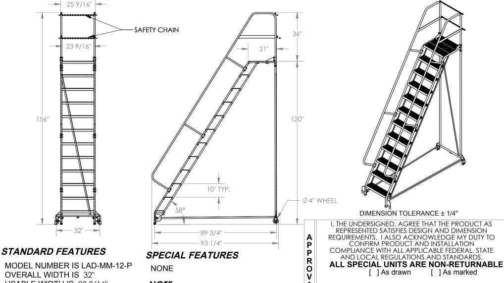
MODEL NUMBER IS LAD-MM-12-P **OVERALL WIDTH IS 32"** USABLE WIDTH IS 23 9/16" **OVERALL LENGTH IS 93 1/4"** USABLE LENGTH IS 89 3/4" **OVERALL HEIGHT IS 156"** PLATFORM HEIGHT IS 120" COLOR: VESTIL BLUE STEP TYPE: PERFORATED STEPS CLIMB ANGLE: 58° STEP DIM. 24" X 7" MAX CAPACITY IS 350 LBS
