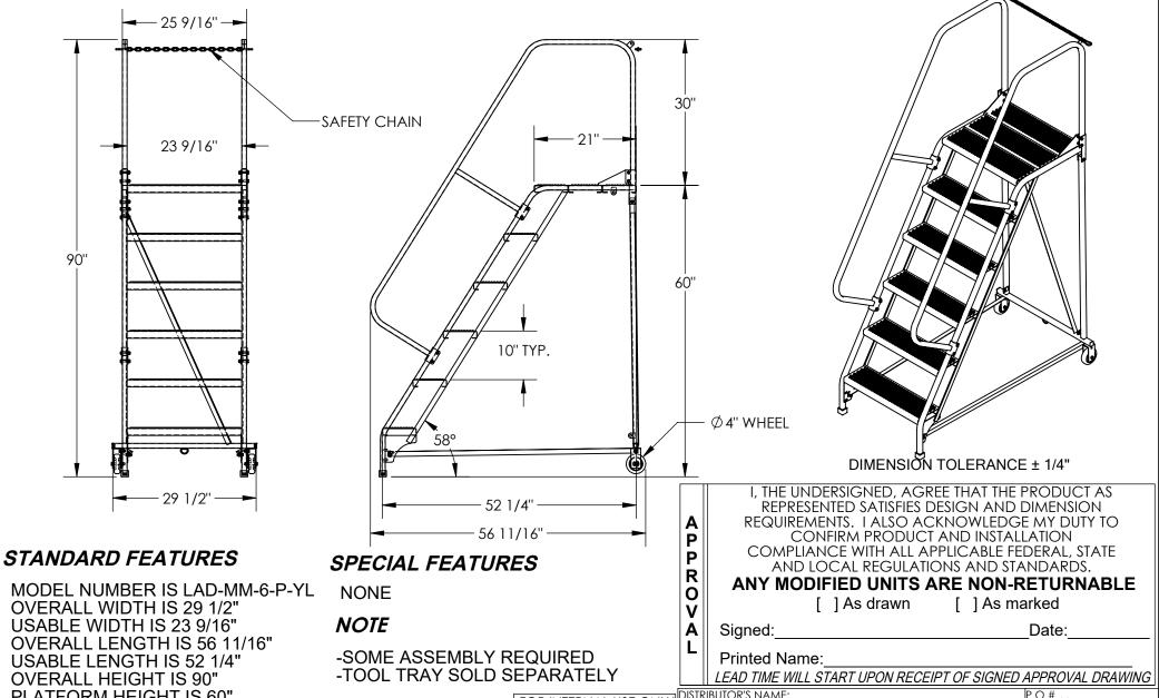
PLATFORM HEIGHT IS 60" TOUGH BAKED IN POWDER COATED YELLOW FINISH STEP TYPE: PERFORATED STEPS CLIMB ANGLE: 58°
