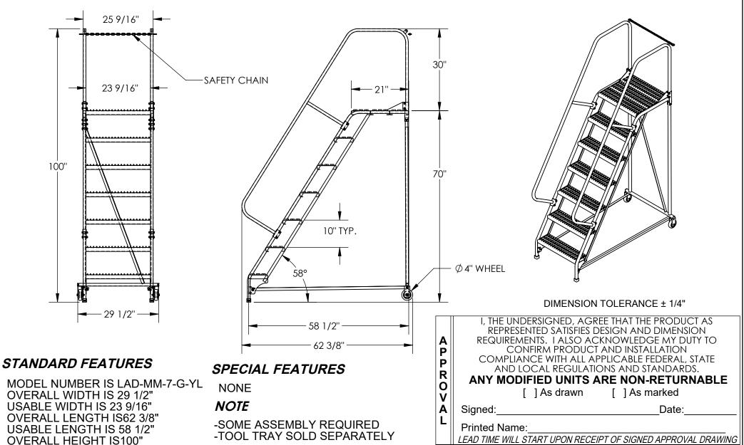
PLATFORM HEIGHT IS 70" TOUGH BAKED IN POWDER COATED YELLOW FINISH STEP TYPE: GRIP STRUT STEPS CLIMB ANGLE: 58° STEP DIM. 24" X 7"
