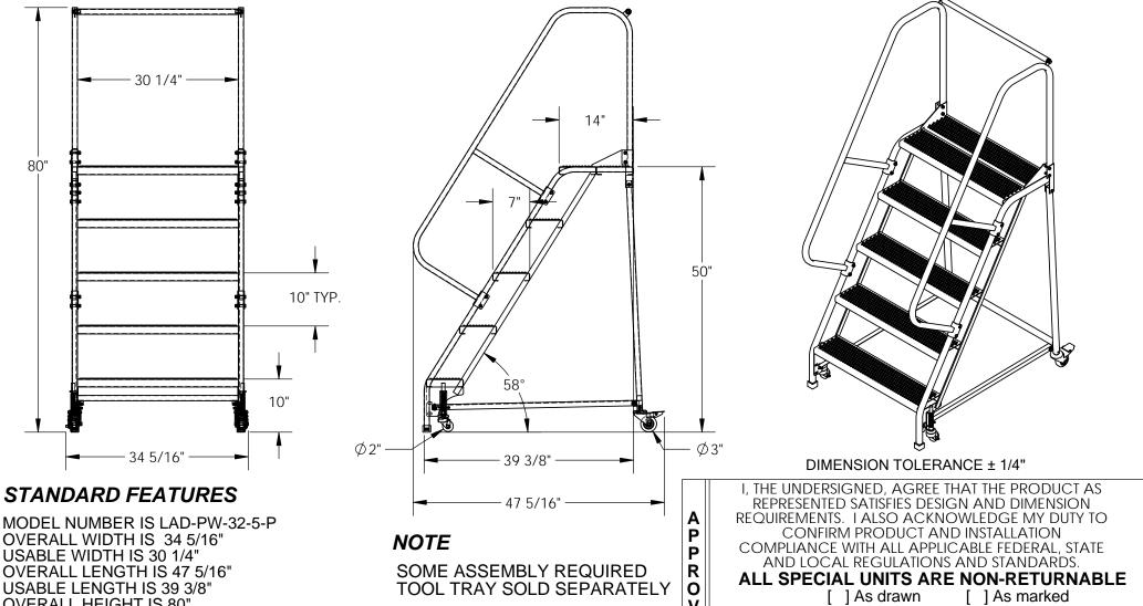
OVERALL WIDTH IS 34 5/16" USABLE WIDTH IS 30 1/4" **OVERALL LENGTH IS 47 5/16" USABLE LENGTH IS 39 3/8" OVERALL HEIGHT IS 80"** PLATFORM HEIGHT IS 50" COLOR IS VESTIL BLUE STEP TYPE IS PERFORATED CLIMB ANGLE IS 58° STEP DEPTH IS 7" PLATFORM DEPTH IS 14" MAX CAPACITY IS 350 LBS
