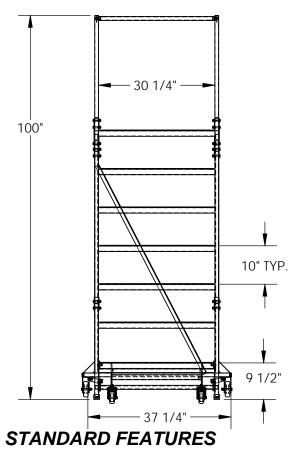
MODEL NUMBER IS LAD-PW-32-7-P OVERALL WIDTH IS 37 1/4" USABLE WIDTH IS 30 1/4" **OVERALL LENGTH IS 56 1/4" USABLE LENGTH IS 51 1/2" OVERALL HEIGHT IS 100"** PLATFORM HEIGHT IS 70" STEP TYPE IS PERFORATED CLIMB ANGLE IS 58° STEP DEPTH IS 7" PLATFORM DEPTH IS 14" **COLOR IS VESTIL BLUE BOTTOM STEP COLOR IS YELLOW** MAX CAPACITY IS 350 LBS FRONT WHEEL IS SWIVEL, SIZE IS Ø 3" REAR WHEEL IS RIGID, SIZE IS Ø 4"
