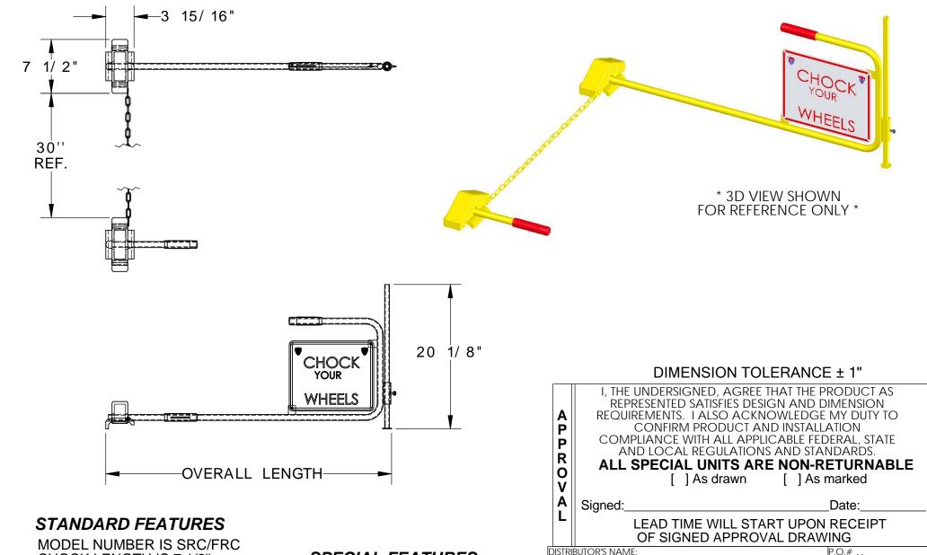
MODEL NUMBER IS SRC/FRC CHOCK LENGTH IS 7 1/2" CHOCK WIDTH IS 3 15/16" OVERALL LENGTH IS 40 5/8" OVERALL HEIGHT IS 20 1/8" COMES WITH SIGN AND LEG 30" CHOCK CONNECTOR CHAIN
