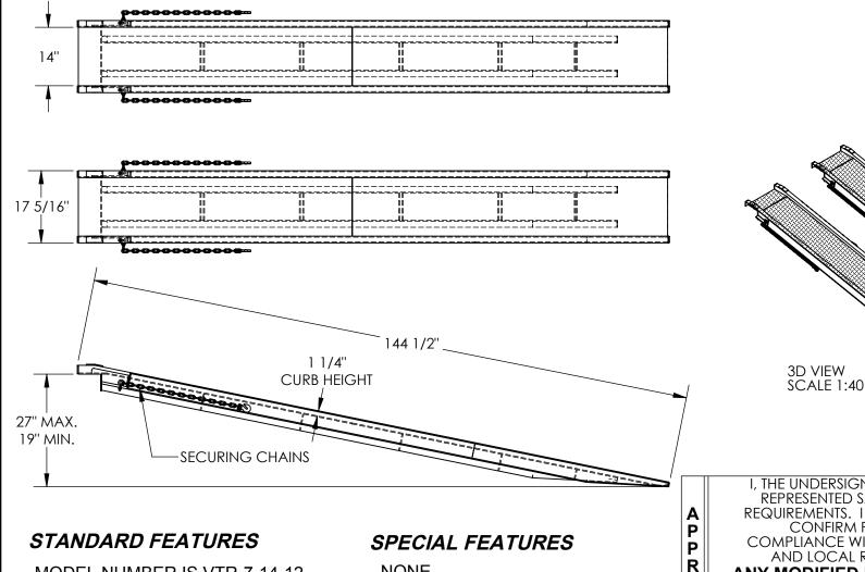
NONE MODEL NUMBER IS VTR-7-14-12 **OVERALL WIDTH IS 17 5/16" USABLE RAMP WIDTH IS 14" LENGTH IS 144 1/2"** MAX. WORKING HEIGHT IS 27" MIN. WORKING HEIGHT IS 19" MAX. LOAD CAPACITY (PER PAIR) IS 7.000 LBS. 1 1/4" CURB HEIGHT **INCLUDES 2 SECURING CHAINS** WELDED ALUMINUM CONSTRUCTION
