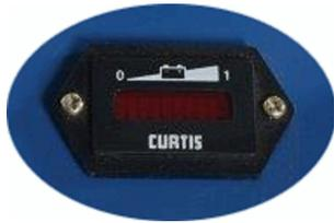
Always check the gauge before using the device; make sure that the battery is charged before using the pallet truck.
