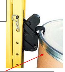
Then move the transporter forward so the lower jaw contacts the metal skirt under the drums locking band and continue to elevate the drum upward. Do not allow the lower jaw to make contact with the paper portion of the fiber drum when trying to elevate the drum.
