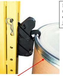
Raise the clamping mechanism until the lower jaw is just high enough to contact the metal skirt just below the locking band.
