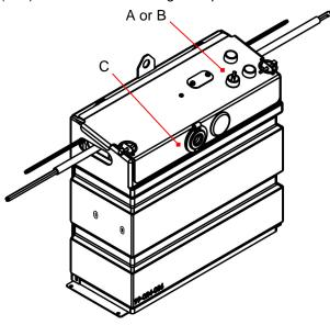
Label 206 (all units; applied to oil reservoir inside power unit housing): Hydraulic oil specifications
