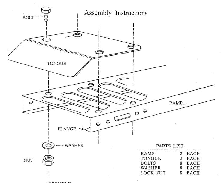
WARNING: ASSEMBLE ONLY AS PICTURED ABOVE AND DO NOT ASSEMBLE WITH THE FLANGE FACING UP. THE FLANGE PROVIDES STRENGTH WHEN FACING DOWN AND IT IS NOT DESIGNED TO FUNCTION AS A TIRE GUIDE.
