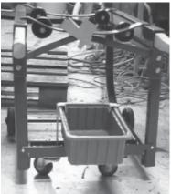
Tilting drip pan forward slightly to clear bracket fingers, slide drip pan into brackets.
