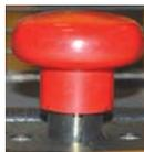
Use E-stop as a service brake to secure the RT-EPT when parked.
