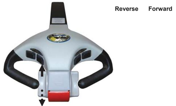
The degree of rotation determines the speed of movement, so the farther you press the wheel in either direction, the faster the S3 will travel, up to a maximum speed of ~3mph when unloaded or ~2.6mph when loaded to capacity. Simply by releasing the movement control, the S3 will decelerate to a complete stop.
