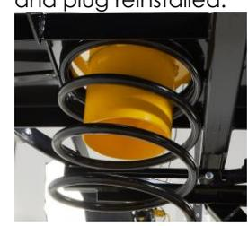
**Step 6:** Make sure that the top of the spring is properly seated inside the upper spring receiver; then remove the clevis pin.
