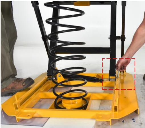
**Step 7:** Press the tabletop down until the latches catch; then pull out the free end of the shock absorber and attach it to the shock bracket using the clevis pin and linchpin.
