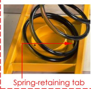
**Step 5:** Compress the spring by pressing down on the second or third loop (not the top of the spring) and slide it under the tabletop.
