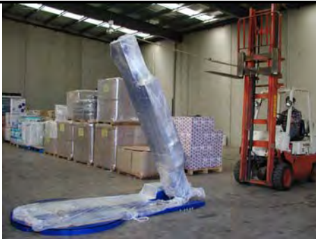
5. Slowly move back the fork lift until the Pillar is up around 80 degree to the ground.
