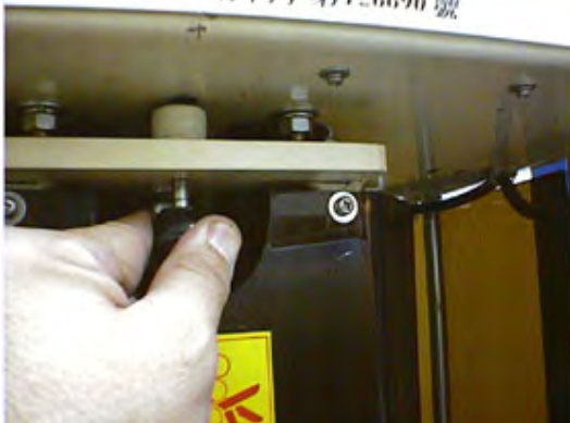
3. Pull down film seat cover lock.
