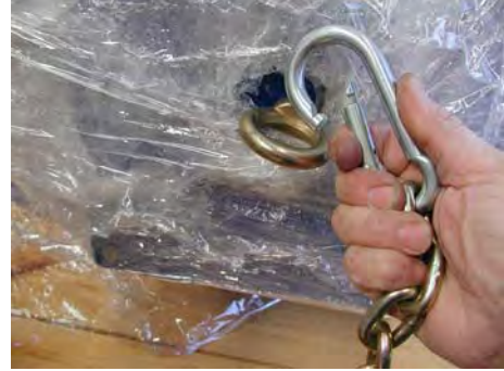
2. Hook the chain on the eye end.
