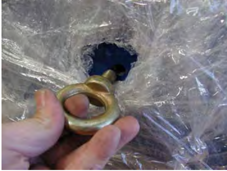
1. First fix an eye end screw on the top of Pillar.
