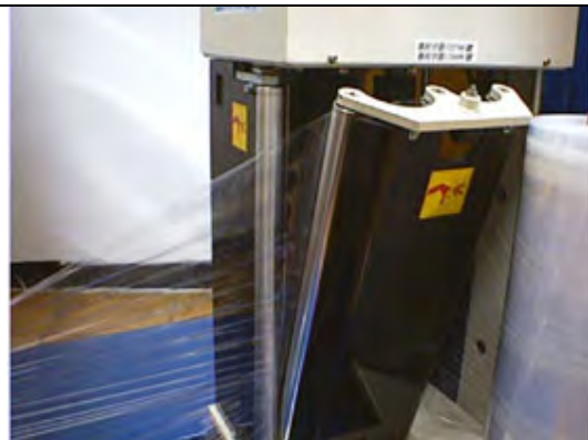
6. Have at least 20-30cm of film out through between film seat cover and rollers.
