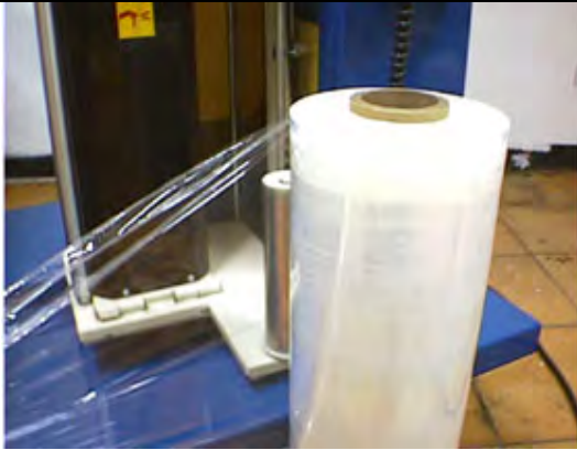
1. Pull out approx. 60cm of film in counter-Clock direction.
