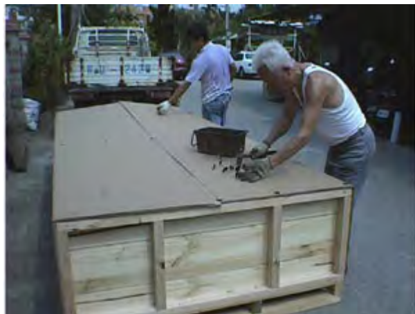
5. Fold the carton to cover the top and fix by nails with plastic washers.
