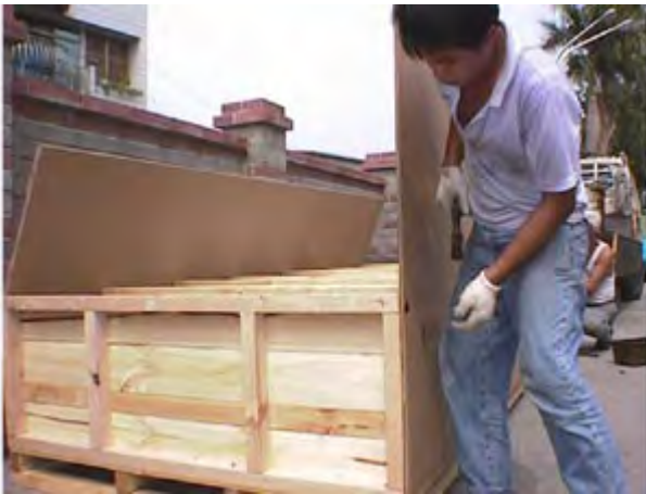
4. Put and fix the side carton.
