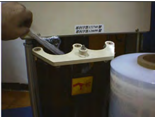
5. Pull out film between film seat cover And film seat rollers.
