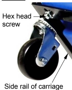
FIG. 1A: Attach casters
