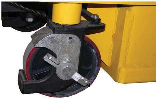
To release the parking brake, press down on the brake pedal
